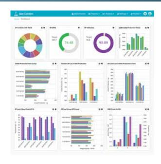
Lap Former LH20 S & Comber LK69 Series can be integrated with Spinconnect, a web based monitoring and control application. The HMI details are transferred through Wi-Fi / LAN Connection and all the parameters can be viewed in a central computer.
