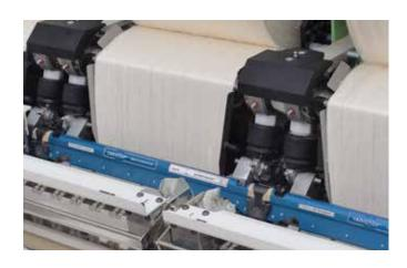
Flexible variocomb with gentle combing facilitates noil removal from 8-25\*%
