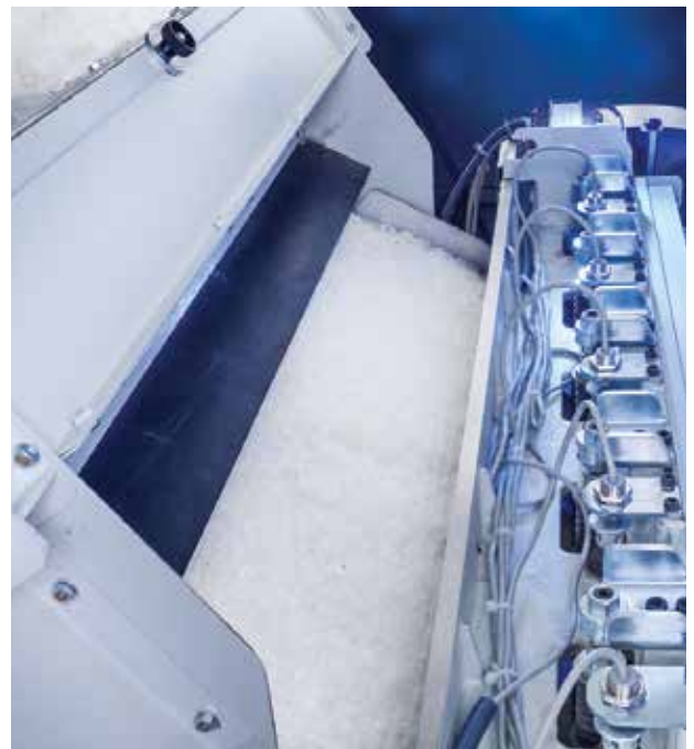
Feed Thickness Measuring System
