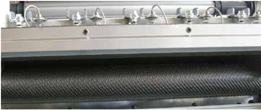
Five Level Sensor Arrangement
